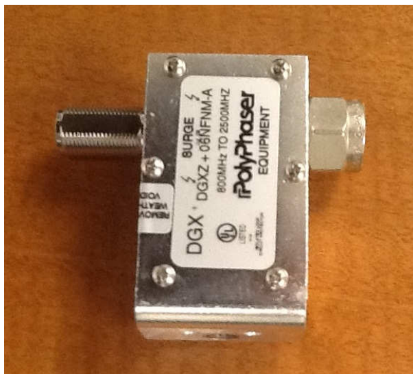
Polyphaser impulse suppressor. Included in kit PN:92-1330 only. Input is on the left and output is on the right. Grounding connection nut is connected on bottom.
