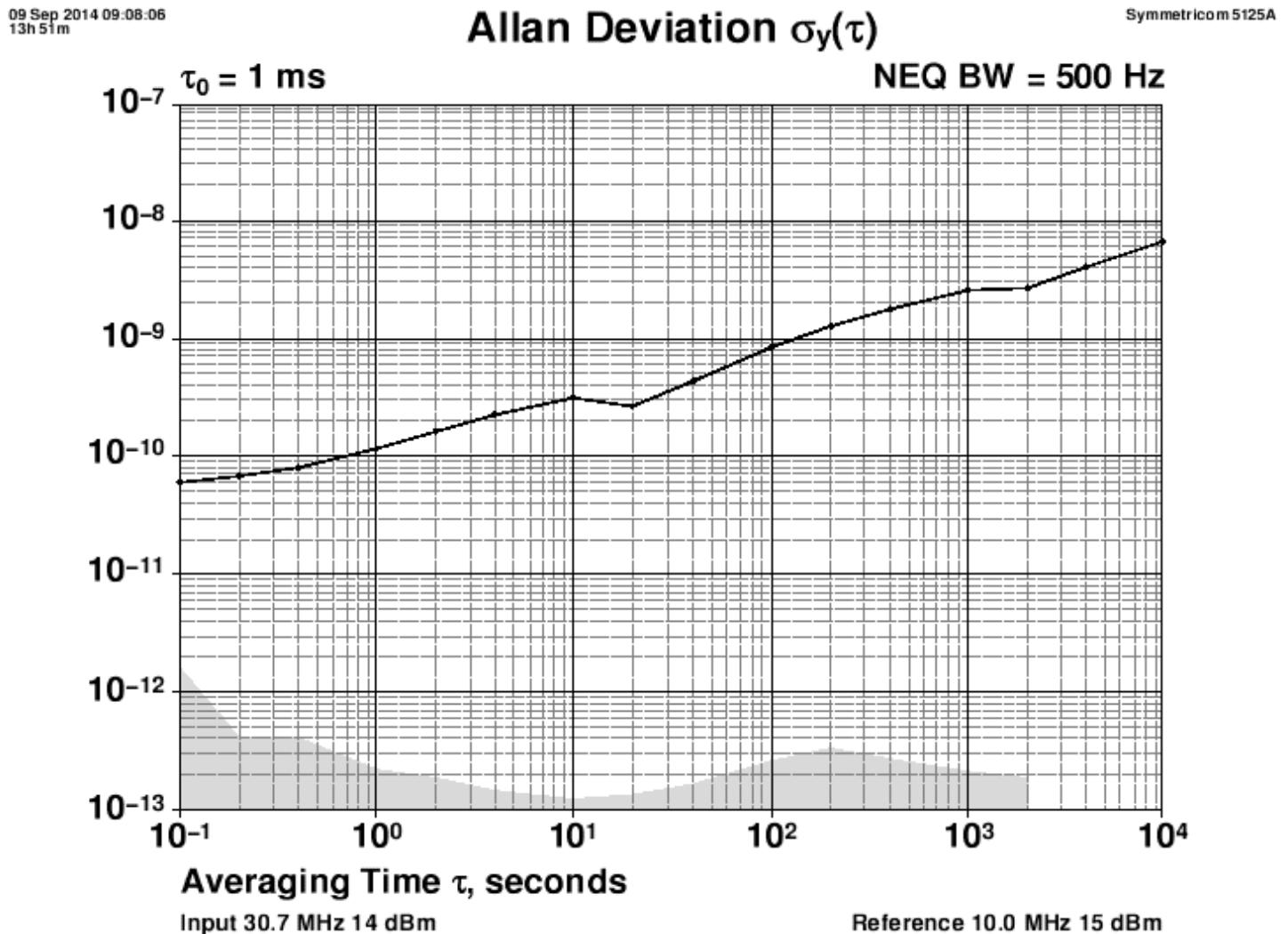
b) LTE-Lite™ ADEV Frequency Drift in holdover (no GNSS)
