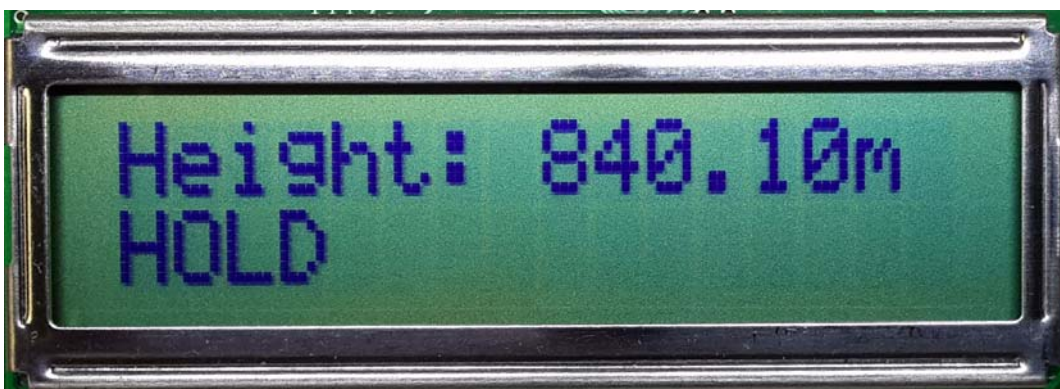
Figure 2.6 GPS height display page
