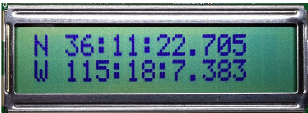
Figure 2.5 GNSS position display page
