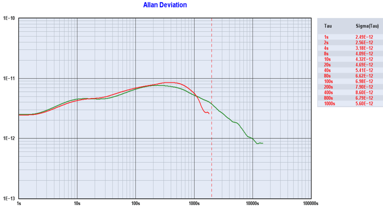
Figure 2.14 Typical Allan Deviation of DROR-II CSAC with double-oven OCXO option
