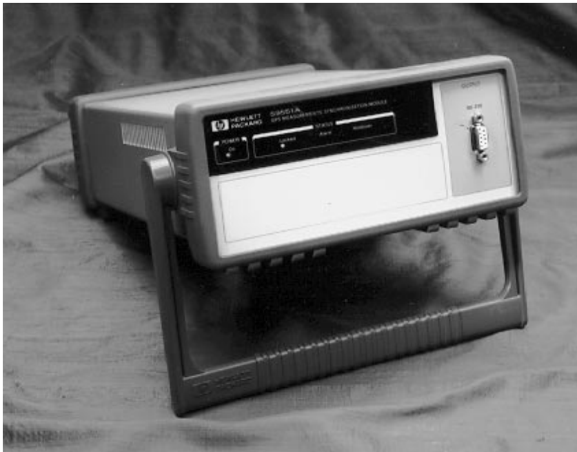
The HP 59551A GPS Synchronization Module is affordable, can be placed at many points throughout a wide-area power system, and provides essential real-time field data for predicting and controlling power system operation.
