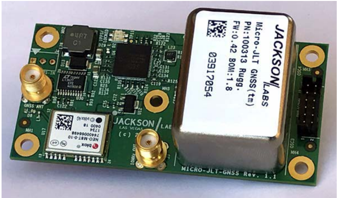
Figure 3 Micro-JLT GNSS™ Double Oven PCB
