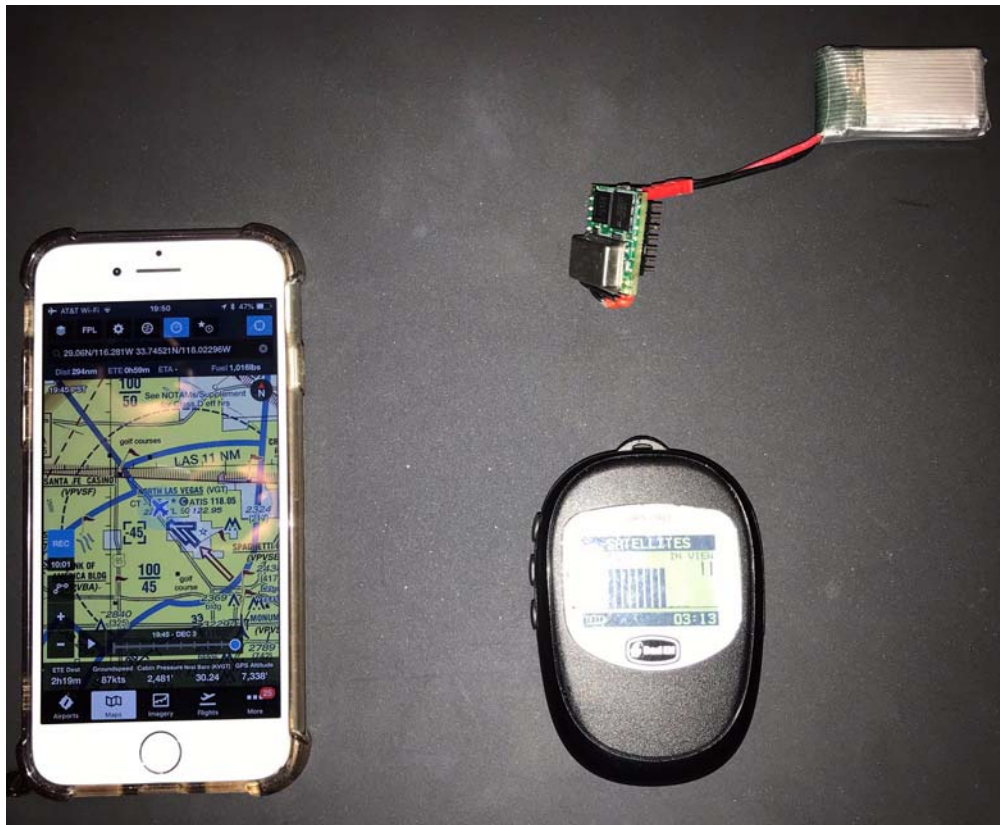
Figure 2.2 Bluetooth GPS Target Receiver with battery-powered Micro GNSS Transcoder™
