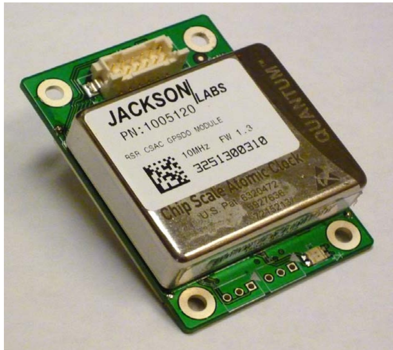
Figure 1.1 Top View of the RSR CSAC GPSDO
